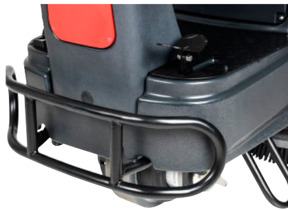
Front bumper protects the machine
